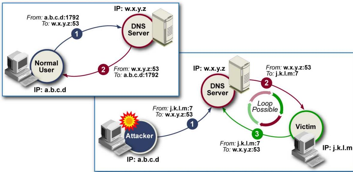
Figure 4-2. Reflector Attack Using a DNS Server
