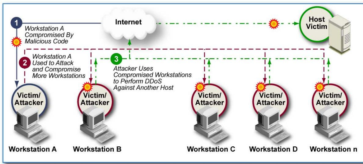
Figure 8-1. Example of a Multiple Component Incident
